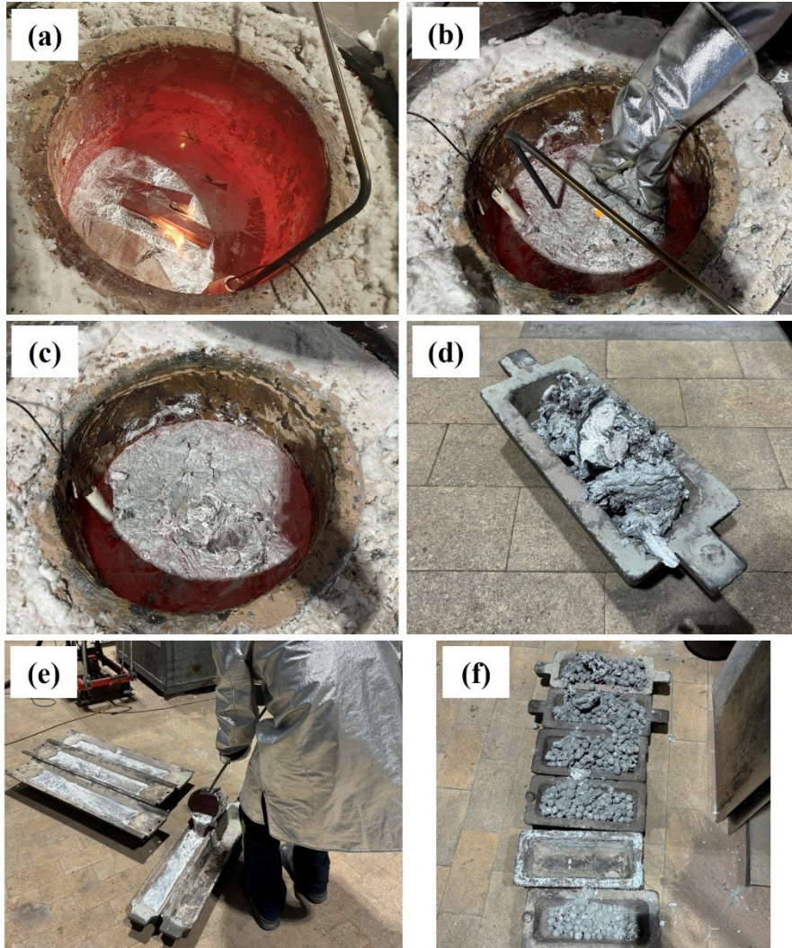
Figure 9. a) Molten aluminium to which the metal pad was added. b) Addition of the metal pad to the molten aluminium. c) Dross formed on the melt. d) Removed dross. e) Tapping aluminium. f) Residual bath and alumina balls.
