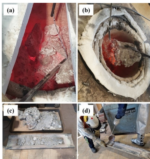
Figure 4. a) Metal pad during melting in crucible at 830 °C. b) Removal of bath residue from crucible. c) Bath residue after test. d) Tapping of aluminium.
